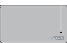
**Data Access:** The red LED indicator will flash while data transmitting.
